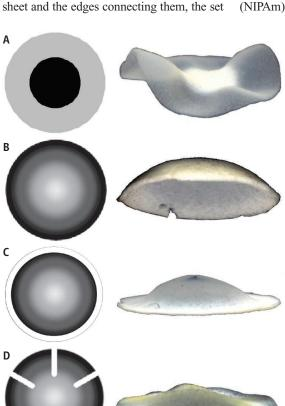
Patterning of cross-linked regions in polymer gel sheets with ultraviolet light creates unequal stresses and drives their buckling into complex three-dimensional shapes.
